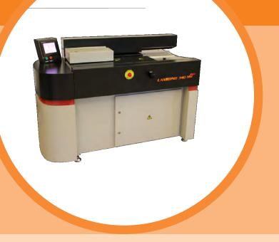
The Rigo LamiBind 340 HM is a semi automatic single clamp perfect binding machine.
